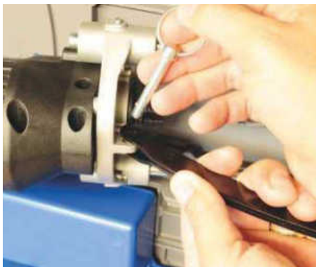
Removing this pin allows the motor to drop out to remove the table
